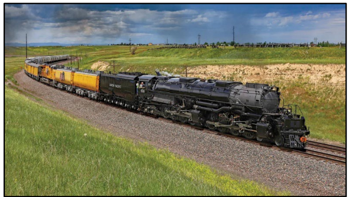
The Big Boy is a 4-8-8-4 articulated locomotive. Photo by Union Pacific Railroad.
